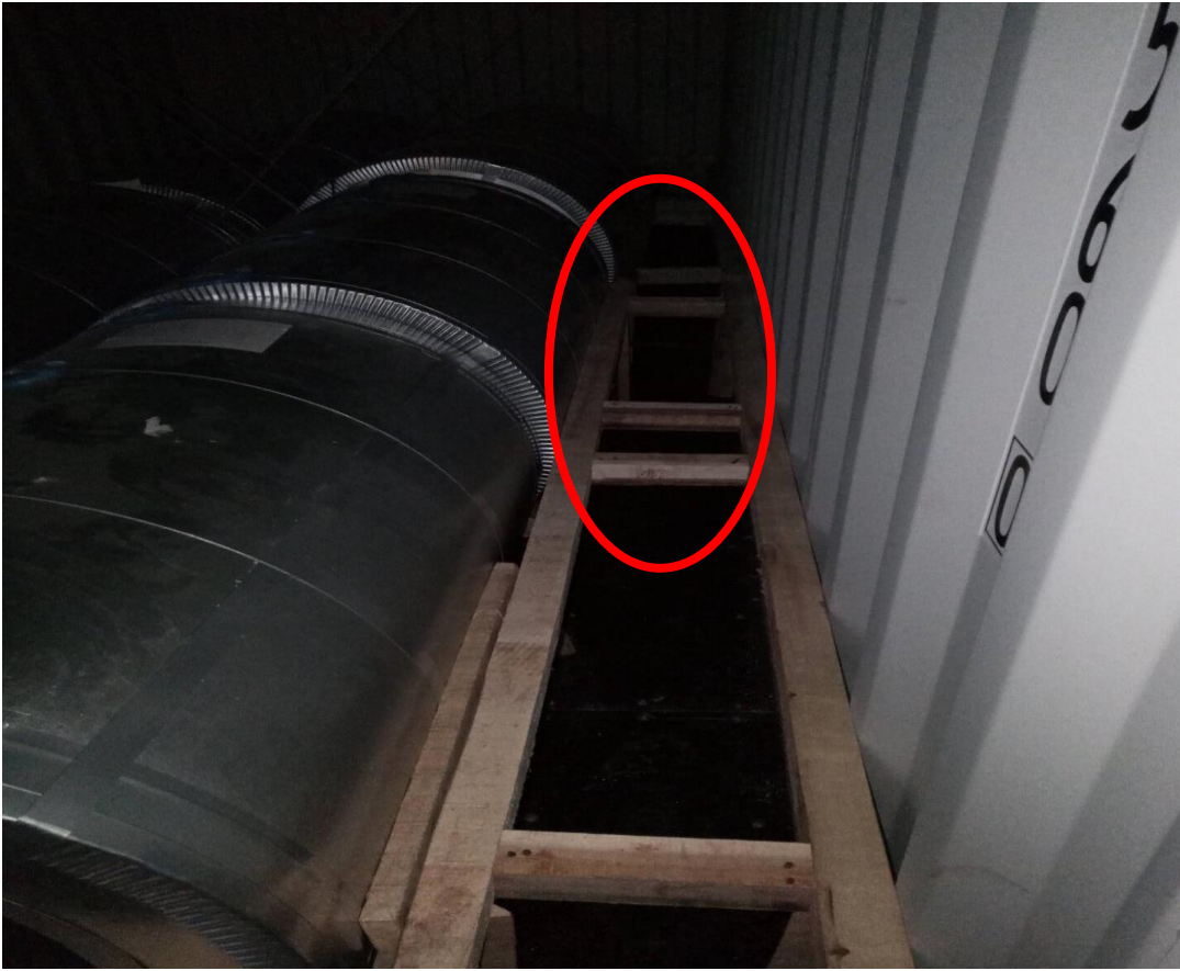
Photo no.3 Last coil in the container is not supposed to touch the container wall
